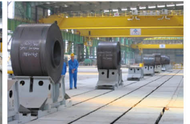
首钢京唐1580mm热轧托盘运输系统 Pallet conveying system for Shougang Jingtang 1580mm hot rolling
