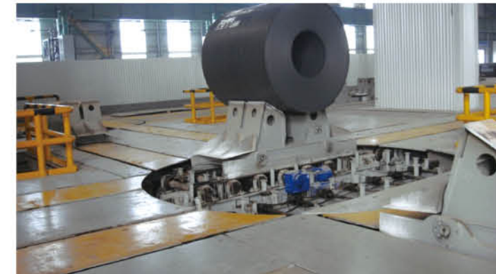
首钢京唐2250mm热轧托盘运输系统 Pallet conveying system for Shougang Jingtang 2250mm hot rolling
