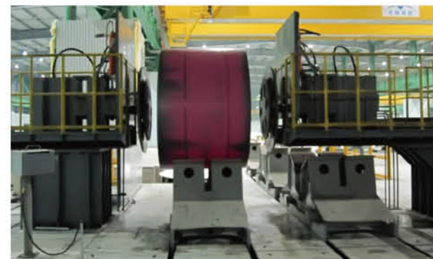
塔形对夹装置（发明专利） Telescopes clamping device (patent of invention)
