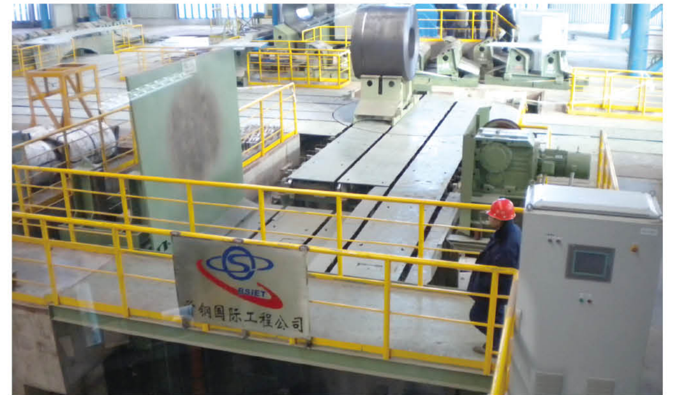
首钢迁钢1580mm热轧托盘运输系统 Pallet conveying system for Shougang Qiangang 1580mm hot rolling
