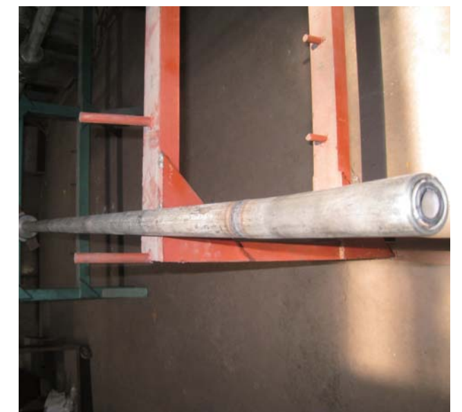
高温耐磨喷枪，使用寿命4-6个月 High-temperature wear-resistant lance, with service life 4-6 months
