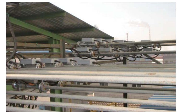
宣钢2号高炉喷煤支管监测 Monitoring of PCI branch pipe for Xuangang 2# BF
