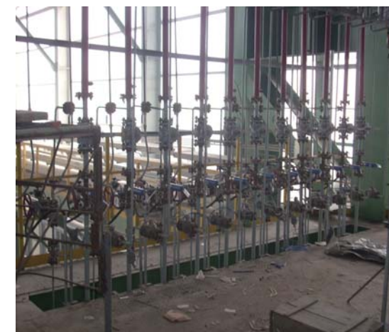
首钢京唐1号高炉喷煤支管监测 Monitoring of PCI branch pipe for Shougang Jingtang 1# BF
