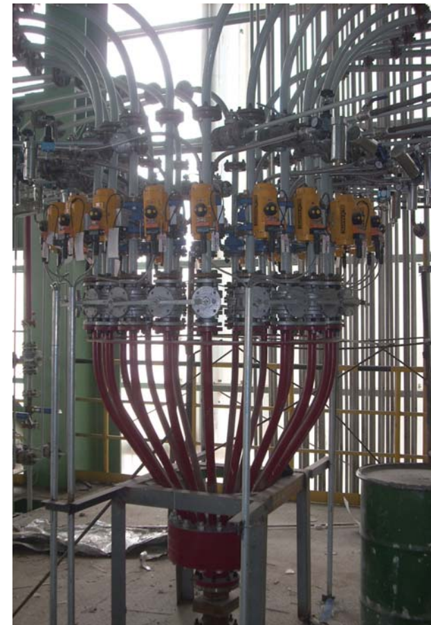
高精度煤粉分配器，每根支管喷煤量更加均匀 High-precision pulverized coal distributor, reaching more uniform coal injection of each branched pipe
