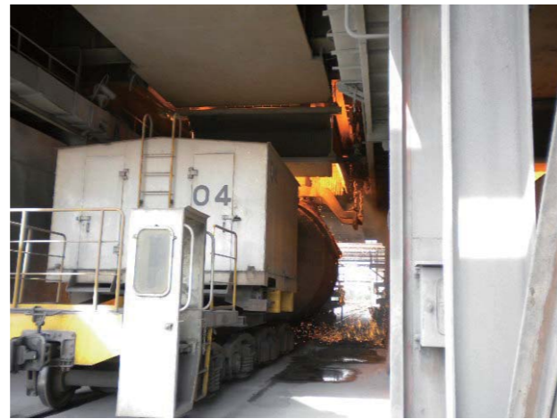
鱼雷罐铁水脱硫 Hot metal desulphurization in torpedo ladle
