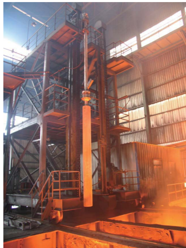
铁水沟铁水脱硫 Hot metal desulphurization in iron runner
