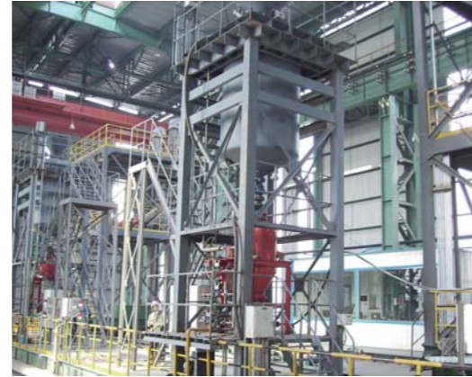
邢钢单吹颗粒镁脱硫设施 Desulphurization by injection of particle Mg only of Xinggang
